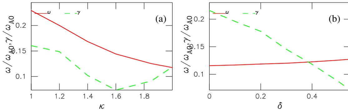
FIG. 4: RKBM frequency and growth rate dependence on plasma cross section ellipticity (figure (a) at  $\delta = 0.49$ ) and triangularity (figure (b) at  $\kappa = 1.85$ ).
