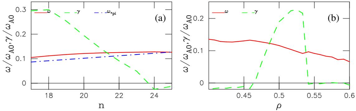
FIG. 3: RKBM frequency and growth rates dependence on toroidal mode number (figure (a),  $\rho = 0.48$ ) and minor radius (figure (b),  $n = 22$ ) for the baseline scenario.
