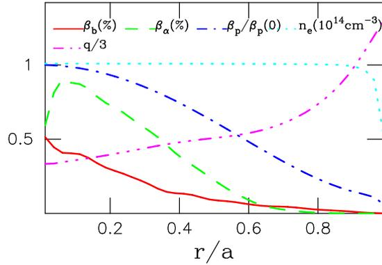
FIG. 1: Plasma profile for ITER normal shear scenario used in HINST simulations. Shown are profiles of beam beta,  $\beta_b$ , fusion product alpha particle beta,  $\beta_\alpha$ , normalized plasma beta  $\beta_p/\beta_p(0)$ , electron density,  $n_e$ , and safety factor scaled by factor  $1/3$ ,  $q/3$ .
