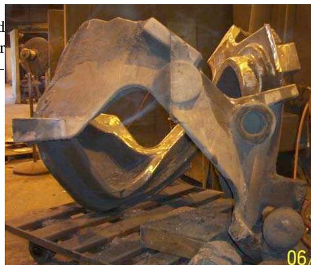
Fig. 5. QPS coil form M1 before machining.
