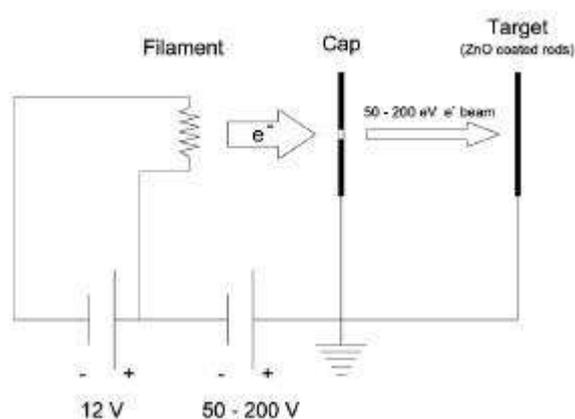
Figure 1. Egun electrical setup
