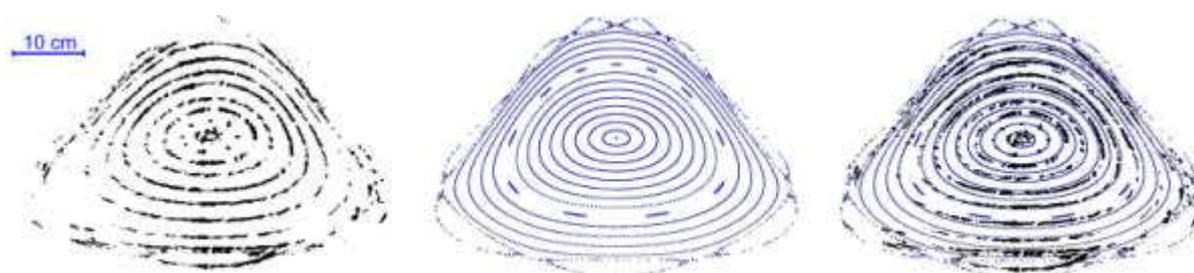
*Figure 3 Left: Nested magnetic surfaces mapped out using a 100 eV e-beam and ZnO coated rods. Middle: Numerically calculated magnetic surfaces plot for 100 eV electrons at 64 angle configuration. Right: The composite image overlaid on the numerical surfaces.*
