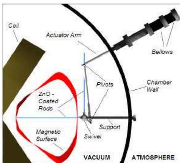
Figure 2. Moveable ZnO coated rod assembly
