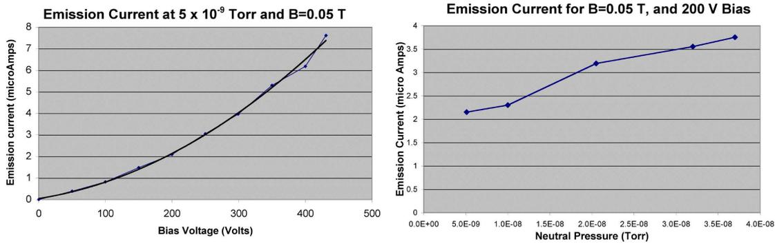
Figure 1: Left: Electron emission rate versus bias for  $B=0.05$  Tesla and a neutral pressure of  $5 \times 10^{-9}$  Torr. Right: Electron emission rate versus neutral pressure for  $B=0.05$  Tesla and a bias of 200 Volts
