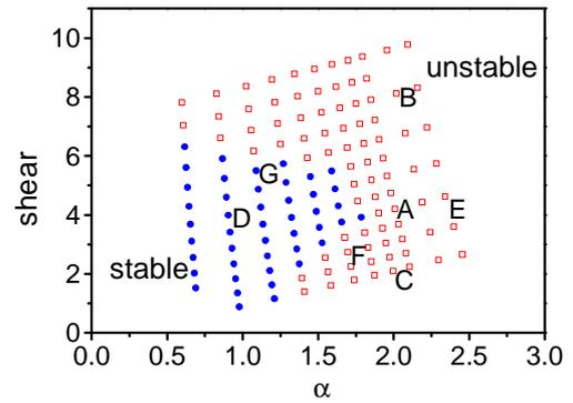
Figure 1. MHD stability of a JET diagnostic optimized configuration shot 55937 just before the type I ELM crash for  $n=6$ . Open squares are unstable points and solid circles are stable ones. The point A corresponds to a reconstruction of experimental equilibrium.
