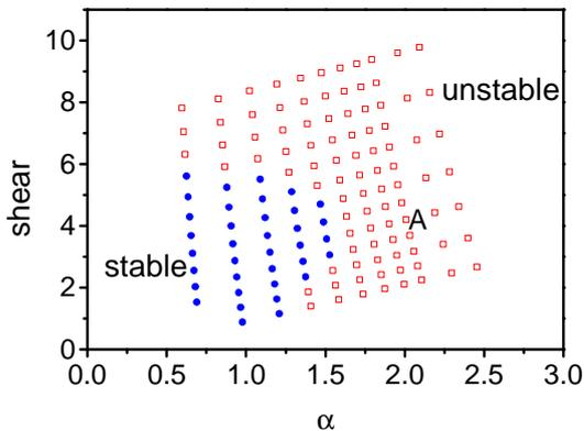
Figure 4. MHD stability of a JET diagnostic optimized configuration shot 55937 just before the type I ELM crash for  $n = 10$ . Squares are unstable points and circles are stable ones. The point A corresponds to a reconstruction of the experimental equilibrium.
