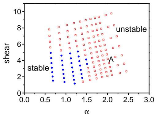
Figure 5. MHD stability of a JET diagnostic optimized configuration shot 55937 just before the type I ELM crash for  $n = 15$ . Squares are unstable points and circles are stable ones. The point A corresponds to a reconstruction of the experimental equilibrium.
