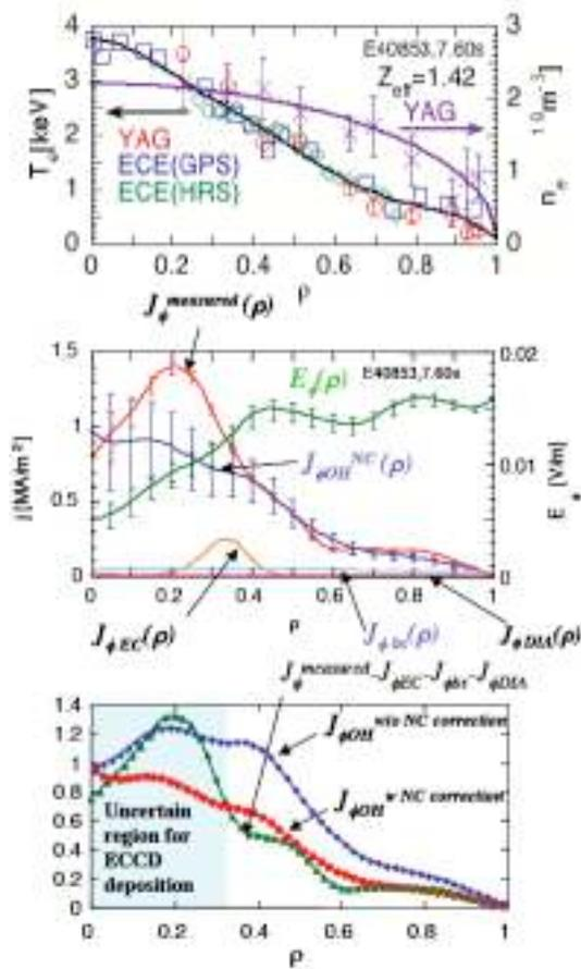
Figure 1  $T_e, n_e$  profiles (top) current density and toroidal electric field profiles. (middle) and comparison of measured and calculated current profiles with and without NC correction to electrical conductivity.
