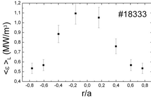
Fig 2. Bolometer line-averaged emissivity
