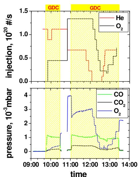
Fig 1: Temporal evolution of the O<sub>2</sub> and He injection rates (upper) and the partial pressures of CO, CO<sub>2</sub> and O<sub>2</sub>. The shadowed areas indicate GDC on/off.
