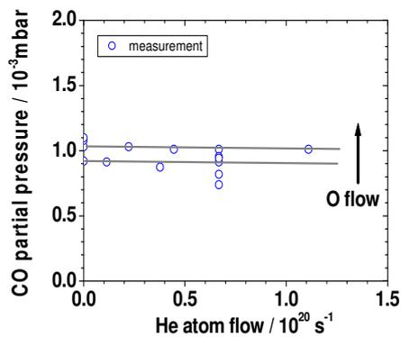
Fig 2: CO partial pressure at different O<sub>2</sub> injection rates depending on the He injection rate.
