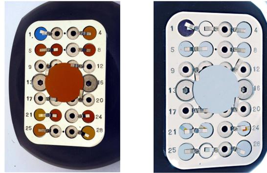
Fig 3: appearance of Si probes coated with a-C:H film before and after O<sub>2</sub> GDC treatment
