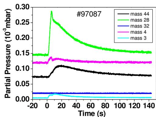
Fig 4: temporal behaviour of CO,  $CO_2$ ,  $O_2$  and HD partial pressure during and after ICRF pulse. The ICRF pulse lasted from 1-3.9 sec and oxygen was injected at 1.1.-4 sec with rate of  $2.1 \cdot 10^{20}/\text{sec}$ .
