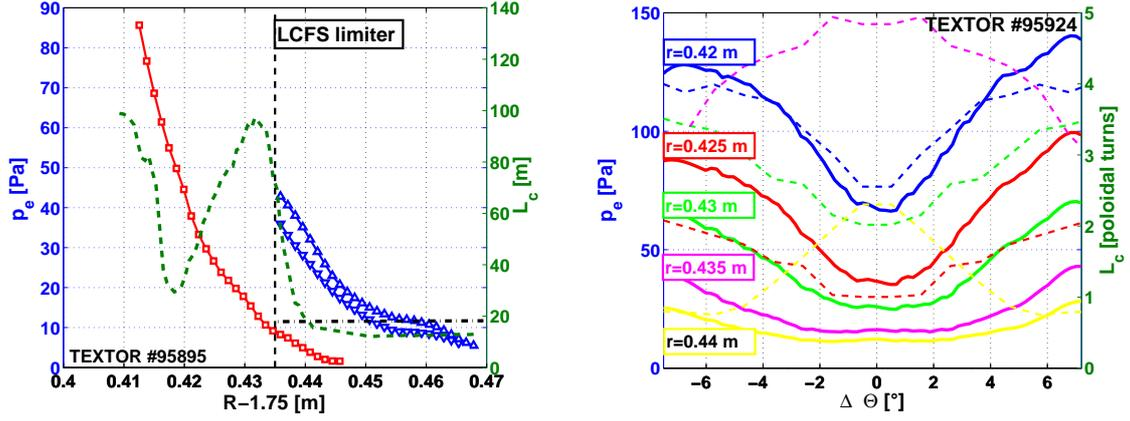
(a) Profiles  $p_e(r)$  with (red line with squares) and without (blue lines with triangles) DED (b)  $p_e(\Theta)$  (solid lines/left abscissa) and  $L_c(\Theta)$  (dashed lines/right abscissa) during sweep
