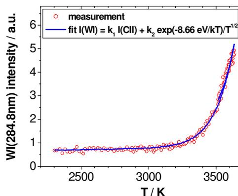
Fig.6 Tungsten flux versus temperature
