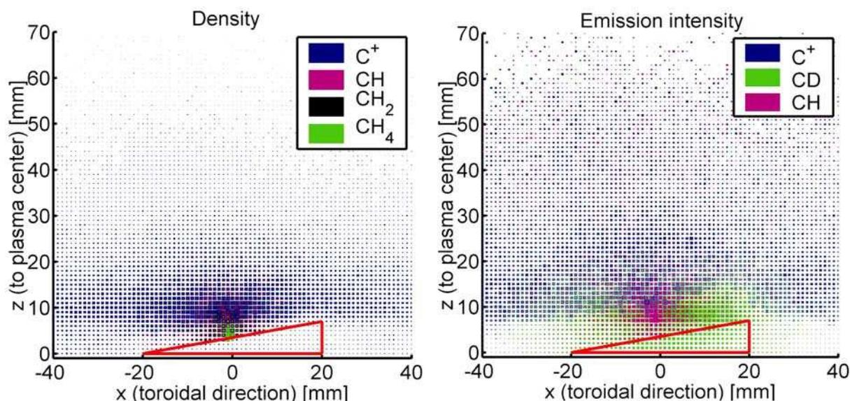
Fig. 2. Distribution of CH<sub>4</sub> and decay products: density (left) and light emission (right) in the observation volume (side view, 20mm nozzle radius,  $\alpha=10^\circ$ ).
