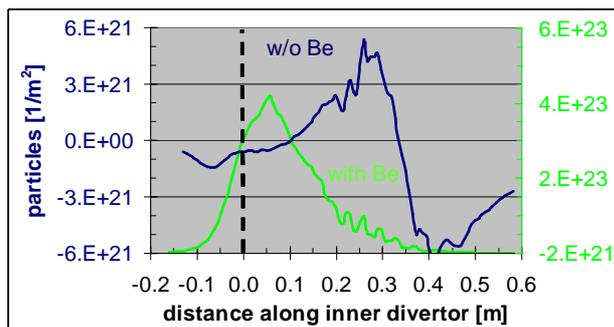
**Figure 4** Profile of net-carbon erosion/deposition after 10s and same profile but with beryllium deposition added.
