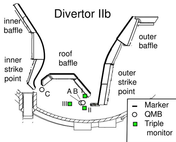
**Fig.1:** Position of diagnostics used in the divertor of ASDEX Upgrade.
