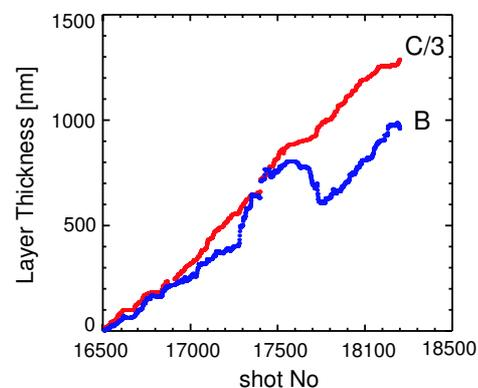
**Fig.3:** Layer Thickness measured by the QMB at outer (A) and inner (C) divertor
