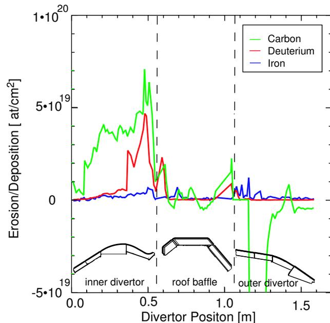
**Fig.2:** Deposition of C,D and Fe found on the poloidal divertor cross section.
