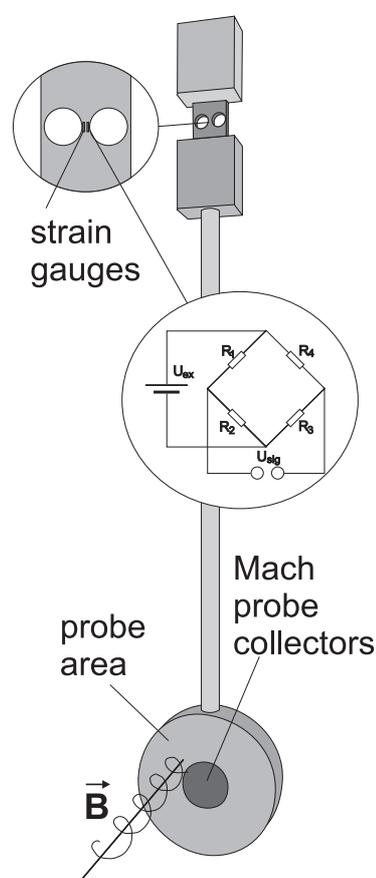
Figure 1: Combined force-Mach-Langmuir probe in a magnetic field
