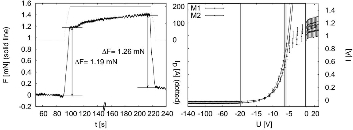
2.a: Force measurement during a plasma discharge
