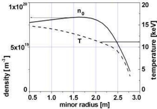
Fig. 2 Stationary profiles of  $n_0(a)$  and  $T(a)$  as functions of minor radius  $a$
