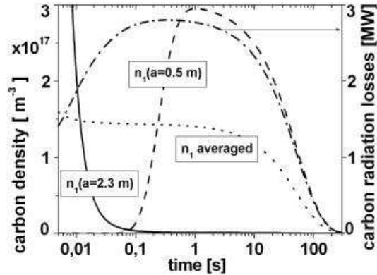
Fig.3 Carbon density and radiation after single ELM of  $j_c = 3 \times 10^{17} \text{ m}^{-2}$
