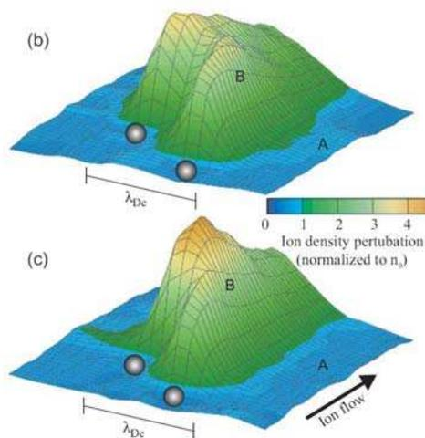
FIG 3. The formation of common wake as particle separation decreasing.
