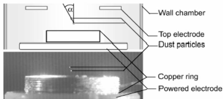
FIG 1. Experimental set-up
