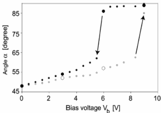
FIG 2. The hysteretic angle  $\alpha$  as a function of the bias voltage  $V_b$ .
