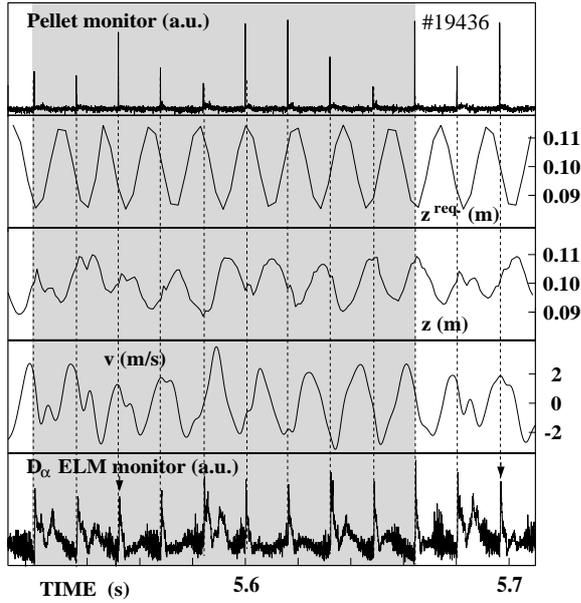
Figure 1: Combination of pellet and magnetic ELM triggering, pellets probing the vertical motion cycle.
