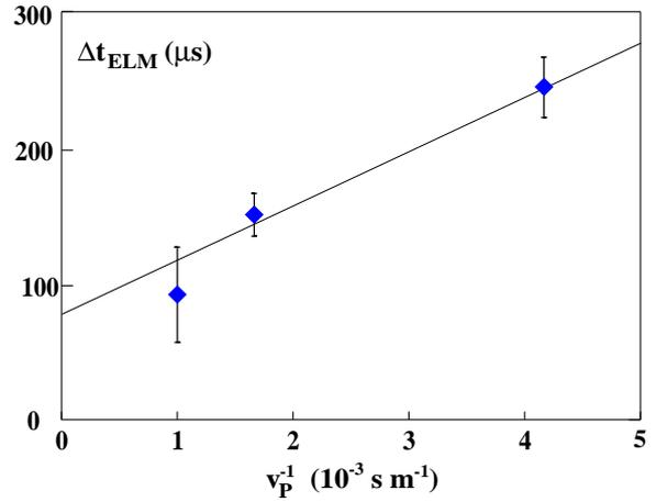
Figure 2: Delay of ELM onset to pellet crossing the separatrix versus inverse pellet velocity. Data indicate for an intrinsic ELM onset time of  $\sim 80\mu\text{s}$ , the ELM trigger seed perturbation is generated  $\sim 40\text{mm}$  inside the separatrix along the pellet path.
