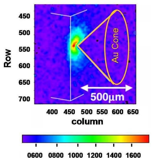
Figure 5: A Au cone has been attached to guide the laser pulse. Electron surface spreading and transport inhibition differs little from the no-cone image.
