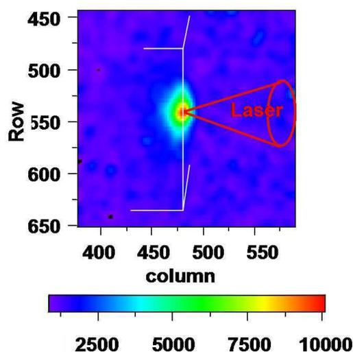
Figure 4: CCD image of Cu  $K\alpha$  from a solid Cu/Al amalgam. At  $53^\circ$  from the laser axis, the image provides a semi-transverse view of the electron flux within the solid.
