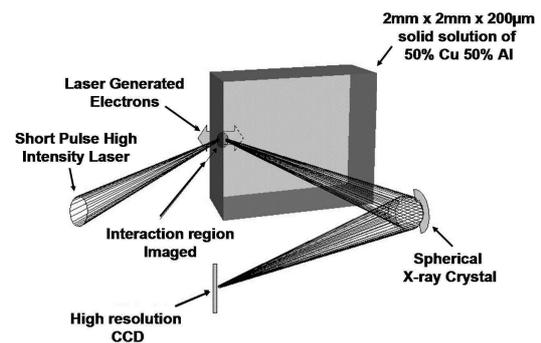
Figure 3: A spherically bent crystal was used to image Cu  $K\alpha$  X-rays from the Cu/Al amalgam onto a CCD.
