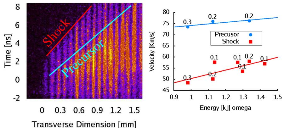
Figure 4: Transverse streak camera
