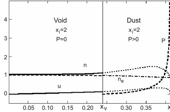
Figure 2: Distributions of the dimensionless parameters in the void and dust regions with the continuous change of the direction of ion flow. The normalized ionization rate is  $x_i = 2$  both in the dust and in the void regions.
