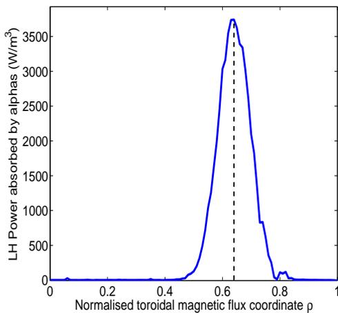
Figure 4: *1D profile of LH power absorbed by alpha particles.*
