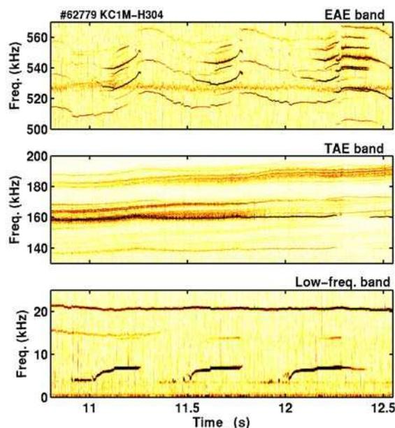
Figure 1. Spectrogram of a magnetic signal in a hybrid JET discharge with  $B=3.2$  T,  $I=2.3$  MA,  $P_{ICRH}=7.6$  MW,  $P_{NBI}=7.8$  MW,  $q_{95}=4.6$ ,  $\beta_N=1.4$ . Sampling rate=2 MHz,  $nfft=8192$ .
