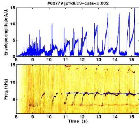
Figure 4. Envelope and spectrogram of  $n=1$  magnetic oscillations. The blue line shows the NTM rotation frequency.
