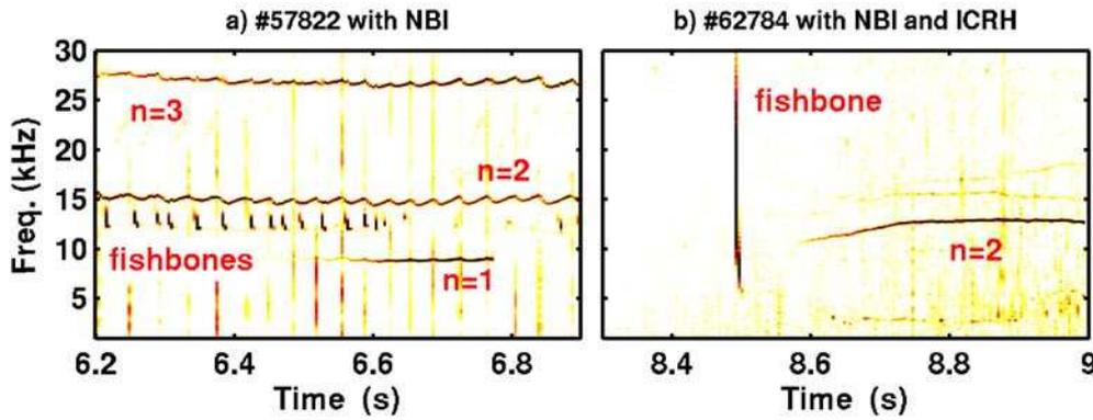
Figure 2. a) Magnetic activity in JET pulse 57822,  $B=1.7$  T,  $I_p=1.4$  MA,  $P_{NBI}=8$  MW, main heating start at  $t=4$  s. b) Pulse 62784,  $B=3.2$  T,  $I_p=2.3$  MA,  $P_{NBI}=8$  MW,  $P_{ICRH}=7$  MW, main heating start at  $t=8$  s.
