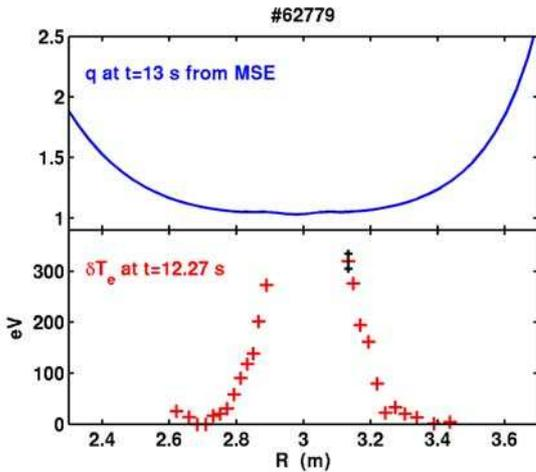
Figure 3.  $q$ -profile and  $n=1$  temperature oscillations from ECE signals. The black segment represents a typical error bar.
