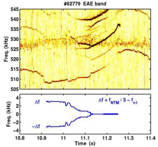
Figure 6. Close-up of the EAE band and difference between  $n=1$  and NTM rotation frequencies. The latter is only shown when the  $n=1$  mode has detectable amplitude.
