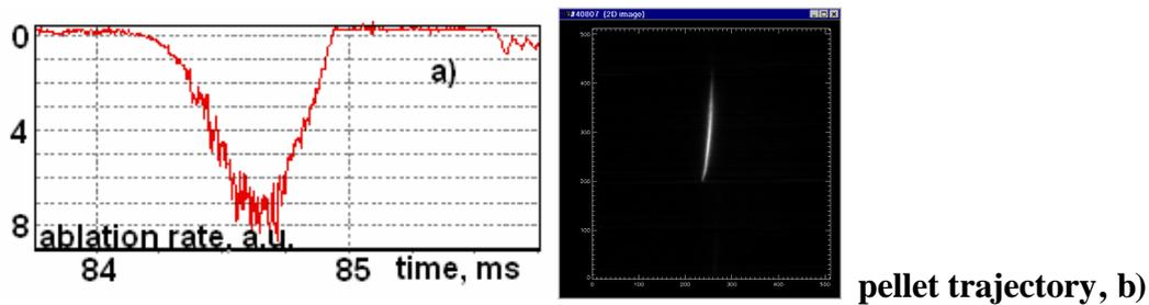
Fig.2. C-pellet, 0.53 mm, 382m/s,  $n(0)=8.2 \times 10^{13} \text{ cm}^{-3}$
