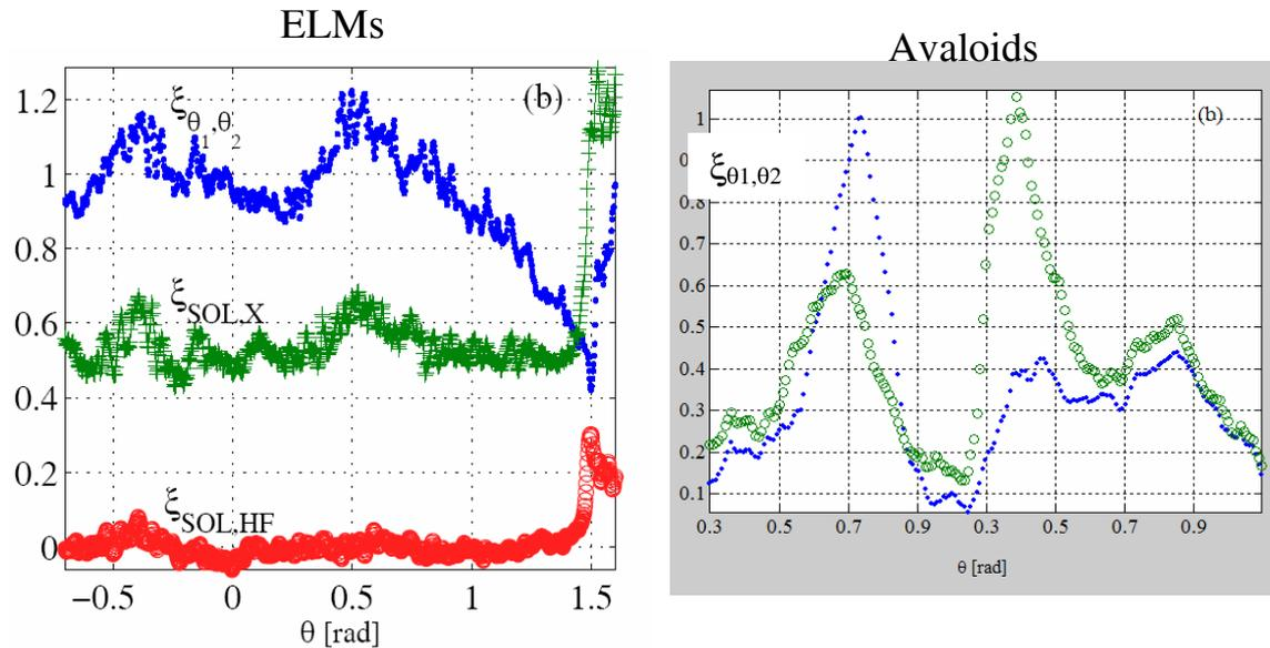
Fig. 3: The slope of the cross-correlation among different points of an image taken from a movie with 300 frames. Note that the cross-correlation is strong at all poloidal angles for ELMs whereas it is localized for avaloids. When the two points are in the SOL, the slope is  $\xi_{\theta_1, \theta_2}$ . When one is in the SOL and the other around the X-point it is  $\xi_{SOL, X}$ , and when they in the low and high field SOL it is  $\xi_{SOL, HF}$ .
