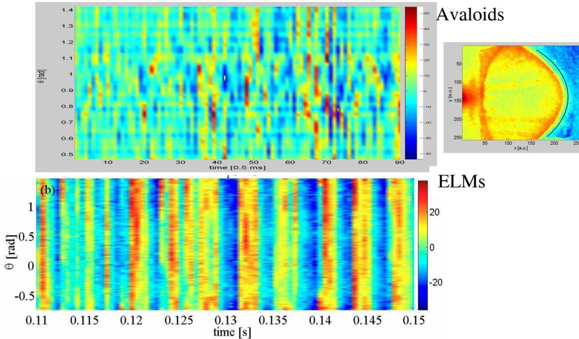
Fig. 2: density fluctuations caused by ELMs (bottom) and avaloids (top) as a function of the poloidal angle and time. The far right-hand image shows a typical image of the plasma with the center stack on the left-hand side.
