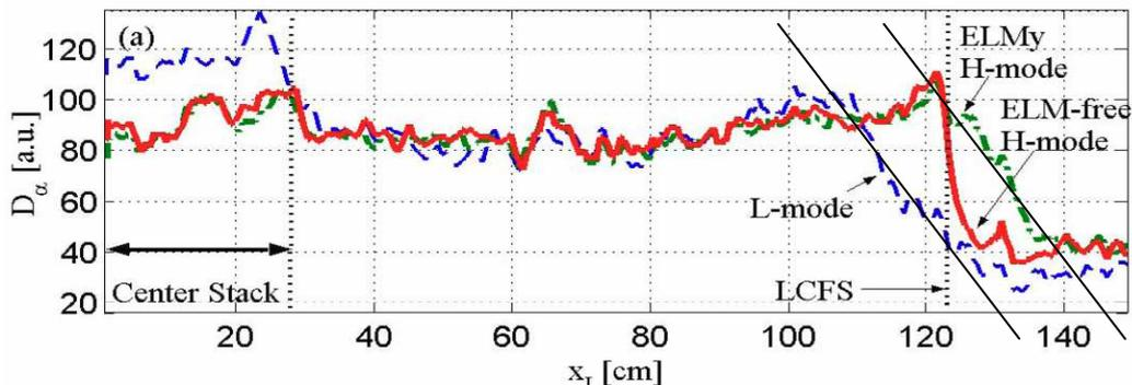
Fig. 4: Radial cut through images of plasma in L-mode (dashed) and H-mode (solid, without ELMs and dash-dotted during an ELM).
