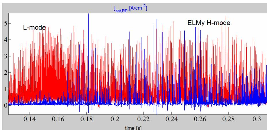
Fig. 1: The ion saturation current as a function of time for two discharges in MAST taken with the same mid-plane Langmuir probe. The probe is approximately at the same distance from the separatrix.
