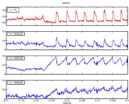
Fig. 1 displays the transition from L-mode to the ELMy H-mode for an  $H_\alpha$  channel and for three neighbouring HCN interferometer channels, one outside of the barrier edge, one at the barrier and one inside the barrier .
