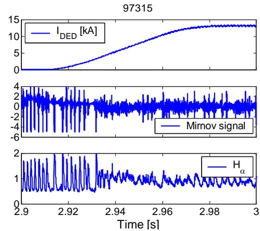
Fig. 4: ELM reduction for increasing DED current.
