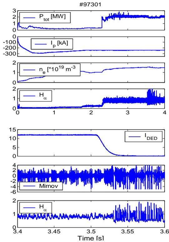
Fig. 3: Different signal channels showing the ELM suppression by the DED. Top figure low time resolution and low figure with higher time resolution.
