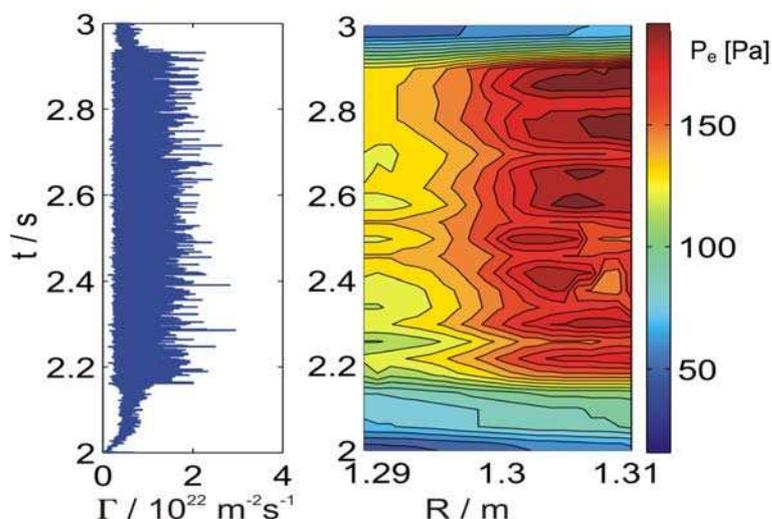
Figure 2: Time trace of the  $H_\alpha$  – signal and the evolution of the edge plasma pressure at the high field side for the TEXTOR discharge # 97315 in false colour technique. The time is represented as ordinate.
