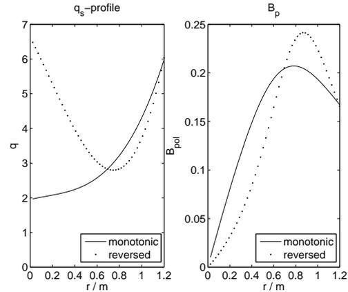
Figure 2: The radial profiles of (a) the safety factor  $q_s$ , and (b) the poloidal magnetic field  $B_p$  for normal (solid line) and reversed (dotted line) configuration.
