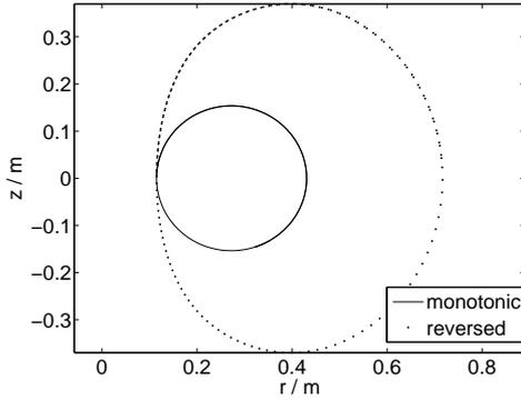
Figure 1: Potato orbits for an 3.5 MeV alpha particle with monotonic (solid line) and reversed (dotted line)  $q_s$ -profile. Due to the smaller poloidal magnetic field in the plasma core, in the reversed case the orbit is significantly wider than in the normal, monotonic case.
