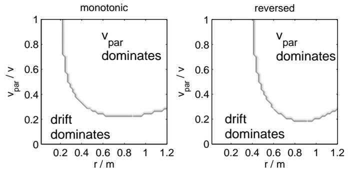
Figure 4: Orbit domains for 3.5 MeV alpha particles with normal (a) and reversed (b)  $q_s$ -profile. The region where gradient drift dominates the particle's natural velocity is on the lower left corner of the plots.
