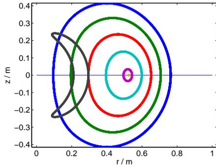
Figure 3: The particle trajectories, calculated by ASCOT [3], for 3.5 MeV alphas with  $v_{\parallel}/v = 0.5$  at the equatorial plane. For comparison, the orbit of a thermal alpha, launched at  $r = 0.3$  m, is also displayed. The remarkable observation is the dramatic shrinking of the orbit width as the alpha particle's birth location moves further away from the magnetic axis.
