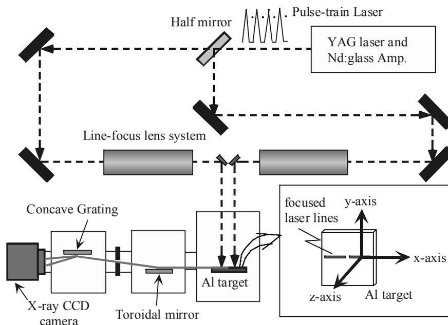
Fig. 1 Schematic drawing of the experimental setup. The coordinate system with respect to the target surface are shown in the inset.
