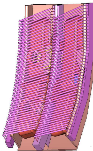
Fig.1. MWS model of half a JET A2 antenna. Left: strap #4 ('outer'); right: strap #3 ('inner'), fed by an in-vessel 'crossover' conductor. Feeders are at a common toroidal location behind strap 4.
