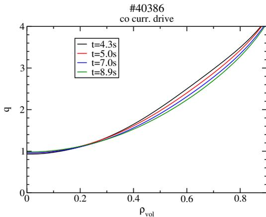
Figure 2: Equilibrium reconstructed  $q$  profile development for off-axis NB co injection (4-9s). The MSE measurement used as constraint for the equilibrium reconstruction do not cover the very centre of the plasma ( $\leq 0.2$ )
