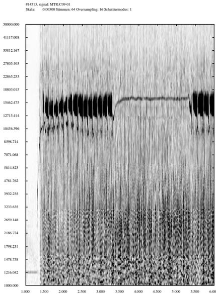
Figure 4: Wavelet plot of the MHD activity in ASDEX Upgrade discharge. The wavelet plot shows the amplitude of a certain MHD activity in darkness, the frequency is on the y axis, and the time is on the x axis. The type of MHD changes with off-axis injection and with turning off the off-axis injection. The mode number and position does not change.
