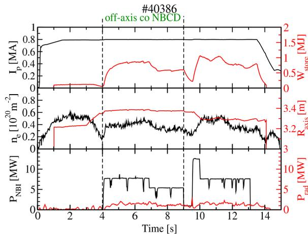
Figure 1: Main time traces for a discharge from JT-60U with strong NB injection in co direction from  $t = 4\text{s}$  to  $t = 9\text{s}$ . In the top graph the plasma current and the stored energy are plotted. In the middle the line integrated electron density (integration length  $\approx 5.2\text{m}$ ) and the  $R$  coordinate of the magnetic axis are represented. Last in the bottom graph the neutral beam injected power and the plasma radiation are drawn.
