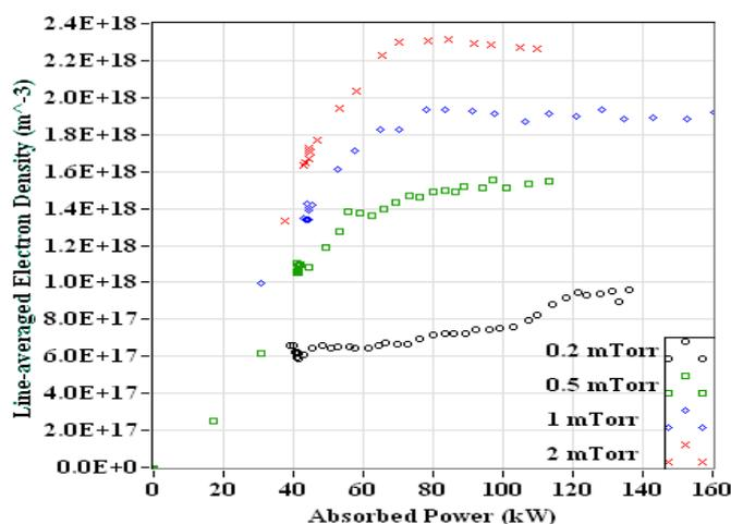
**Figure 5.** Line-averaged plasma density versus absorbed power for different argon neutral pressures.
