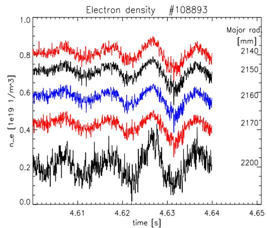
Fig. 6. Time traces of the electron density at different radial positions.
