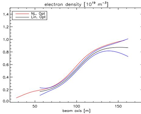
Fig. 5. Electron density profiles reconstructed from the measured  $\text{Li}2p$  intensity profiles shown in Fig. 4. Red curve - from the CCD image, black curve - from the APD measurements. The blue curves is the reliability range ( $\pm \sigma$ ) of the density profile reconstructed from the APD measurement.
