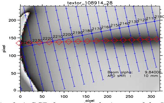
Fig. 1. A CCD frame with the image of the Li beam. The red diamonds mark the positions of the APD channels.
