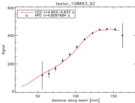
Fig. 4. The  $\text{Li}2p$  line intensity profile along the axis of the Li beam determined from the CCD image (red curve) and from the APD signals (black dots). The error bars indicate the statistical error of the measurements.
