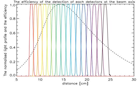
Fig. 2. Uncalibrated sensitivity of the APD channels (colored curves) along the beam axis.
