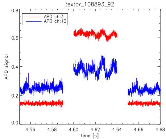
Fig. 3. Time traces of the measured Li2p line intensity for two APD channels.
