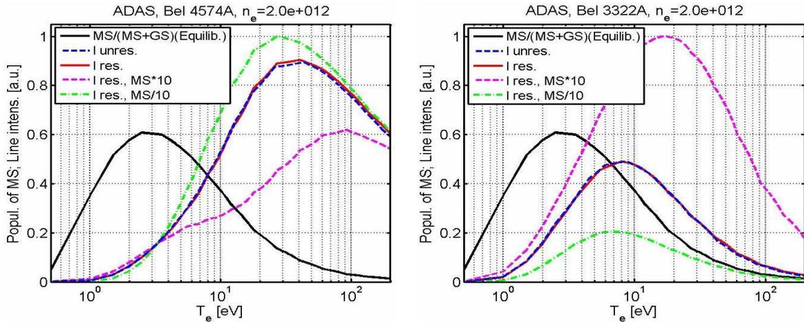
**Fig.3.** ‘Equilibrium approach’ illustration: relative MS population and respective line intensities in MS resolved (“I res.”) and unresolved (“I unres.”) cases; singlet (left) and triplet (right) lines.
