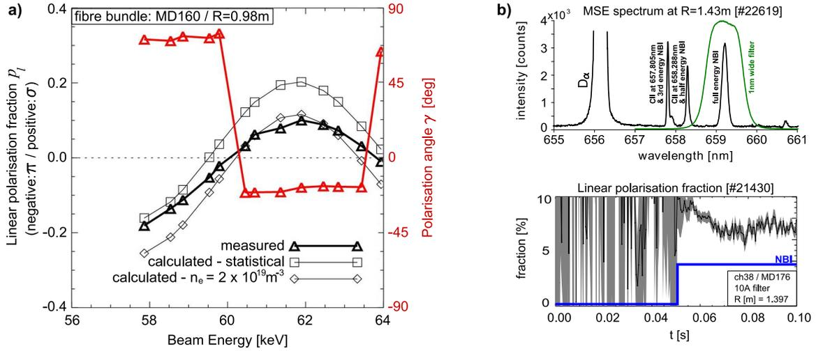
**Figure 1:** (a) Comparison of MSE spectrum simulation with beam voltage scan measurements. (b) Measured polarisation fraction of 7% remains when integrating over the whole spectrum using a 10 Å wide filter.
