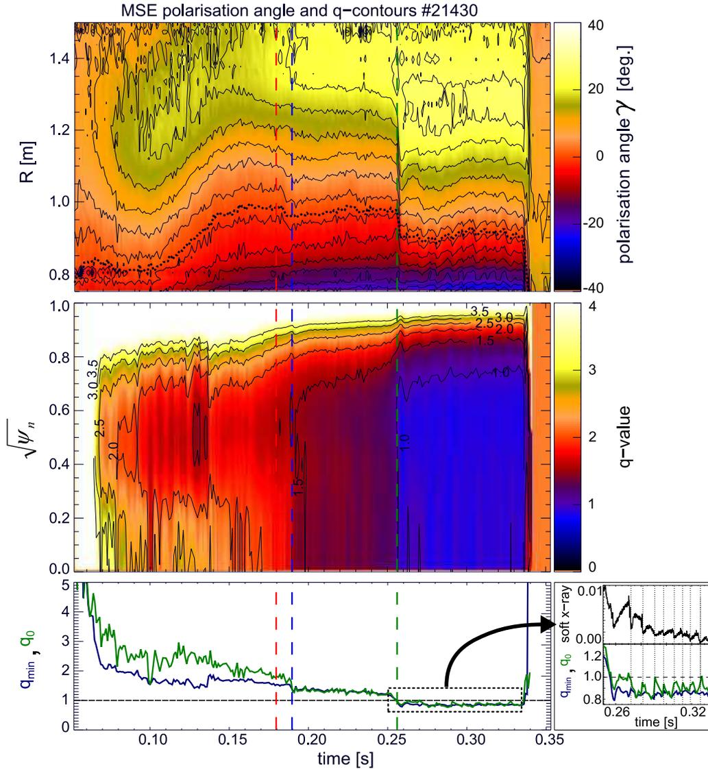
**Figure 2:** Contour plot of the polarisation angle  $\gamma$  measured by MSE and the  $q$ -profile calculated using MSE-constrained EFIT. (MAST discharge #21430).
