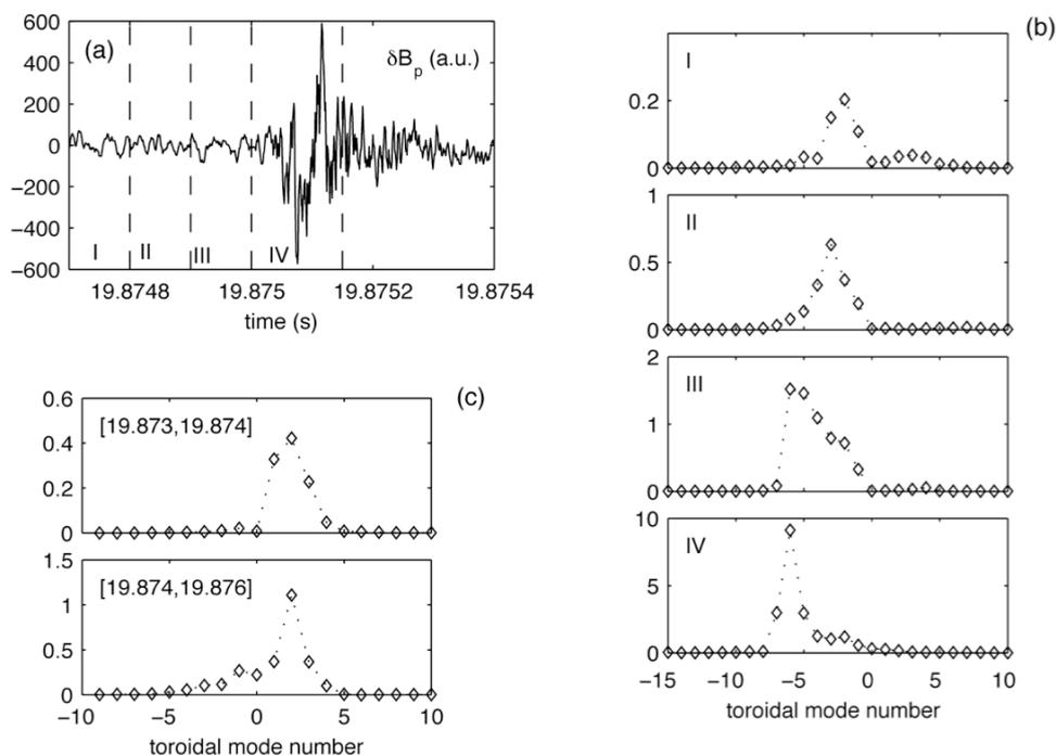
Figure 4. JPN 59423. Pellet-triggered event in H-mode (same event shown in Fig. 3). (a) Magnetic perturbations. Toroidal mode number spectrum associated with components with frequencies  $f < 4$  kHz (b) and with frequencies  $f > 4$  kHz (c).
