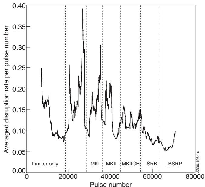
The early attempts were prone to vertical displacement events (VDEs) resulting in a large number of disruptions. A similar period with a high number of disruptions is found during the times leading up to the DT campaign when many of the high power and high current scenarios for these experiments were being developed. Less well explained is the much lower disruption rates observed in the recent campaigns, where after 2001 (#54345) the disruption rate drops significantly below 10%.
