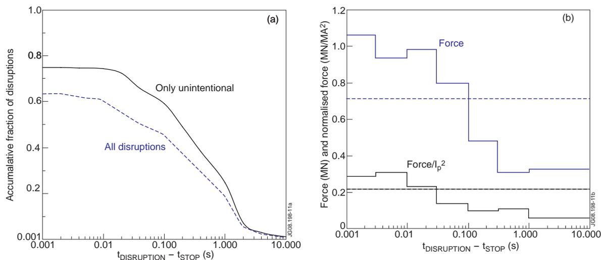
**Figure 3:** **a)** The accumulated fraction of all JET disruptions between 2000 and 2007 (blue dashed) and only unintentional ones, as function of the warning time, i.e. the time between a possible pulse termination trigger and the disruption. **b)** The averaged vessel force (blue) and normalised force for disruptions (black) versus the warning time. The dashed lines gives the force averaged over all disruptions (= 0.71MN) and the average normalised force (=0.218MN/MA<sup>2</sup>).
