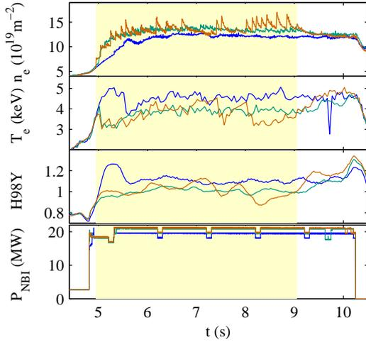
Fig 4 Density, confinement factor (H98Y) and injected power for three discharges: 77858 (blue) reference discharge, #77863 (green) LFS pellets, #77864 (red) VHFS pellets.
