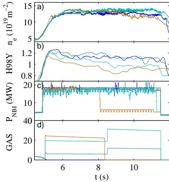
Fig 1 (a) Line integrated density; (b) H98Y confinement factor; (c) neutral beam power (d) and the injected gas level for four discharges: #75954 (blue), #75962 (green, GIM 8), #76748 (red GIM 8), #76749 (cyan GIM 11).
