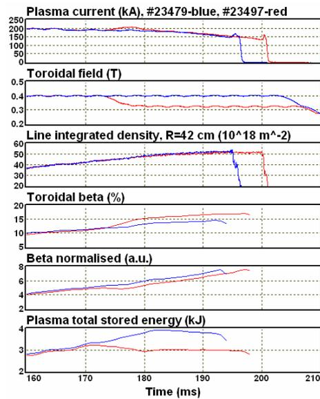
Fig. 3. High density OH shots with (#23497) and without (#23479) toroidal field ramp down.
