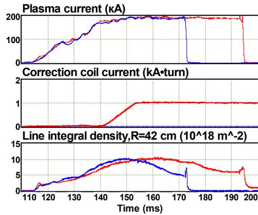
Fig. 2. OH shots with (#22632) and without (#22633) error field correction coils.
