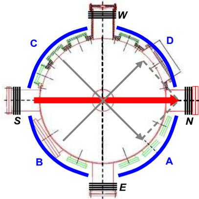
Fig. 1. Globus-M top view with resulting magnetic field (→) produced by two pairs of error field correction coils (A,C) & (B,D).
