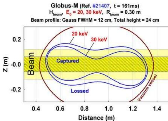
Fig. 5. Simulated regions of orbital losses of beam particles, mapped on the vertical cross section of Globus-M along the NBI direction.
