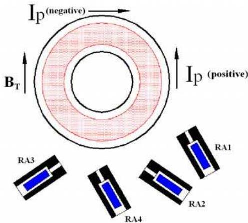
Fig.1 Schematic view of runaway electron diagnostics (down view); RA1(CdTe); RA2(CdTe); RA3(NaI); RA4(NaI)
