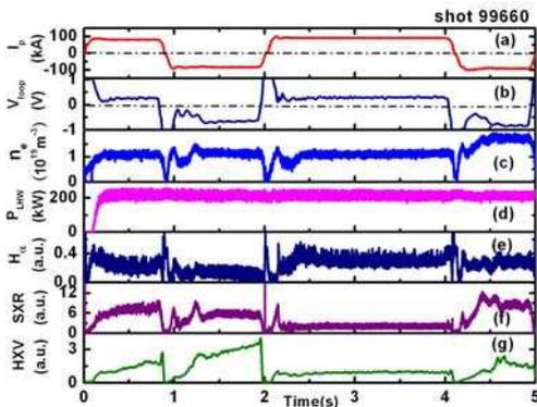
Fig.5 Typical AC discharge (shot No.99660) with LHCD
