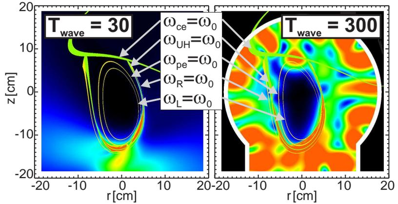
Figure 2: Full-wave simulation with IPF-FDMC for an X-mode incident from the bottom; left part without, right part with vacuum vessel included in the calculations.
