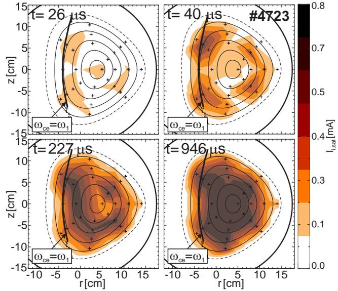
Figure 1: Plasma breakdown as time series for a hydrogen discharge.
