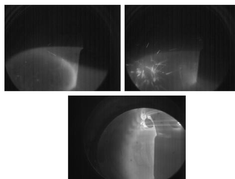
Figure 5: Images from the fast camera in the visible range – flat-top phase, and plasma disruption
