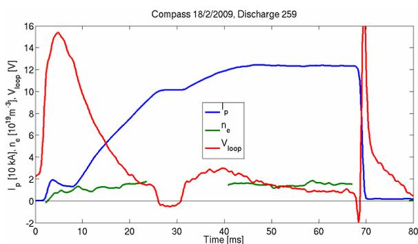
Figure 4: Temporal evolution of the loop voltage, plasma current and the line average density .
