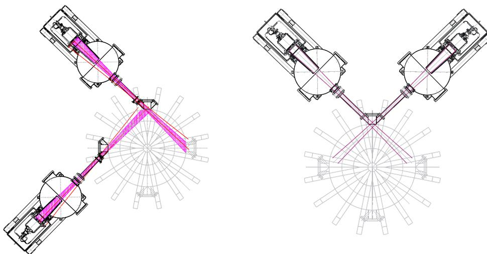
Figure 3: Top view on the NBI system layout. Left: co-injection, right: balanced injection
