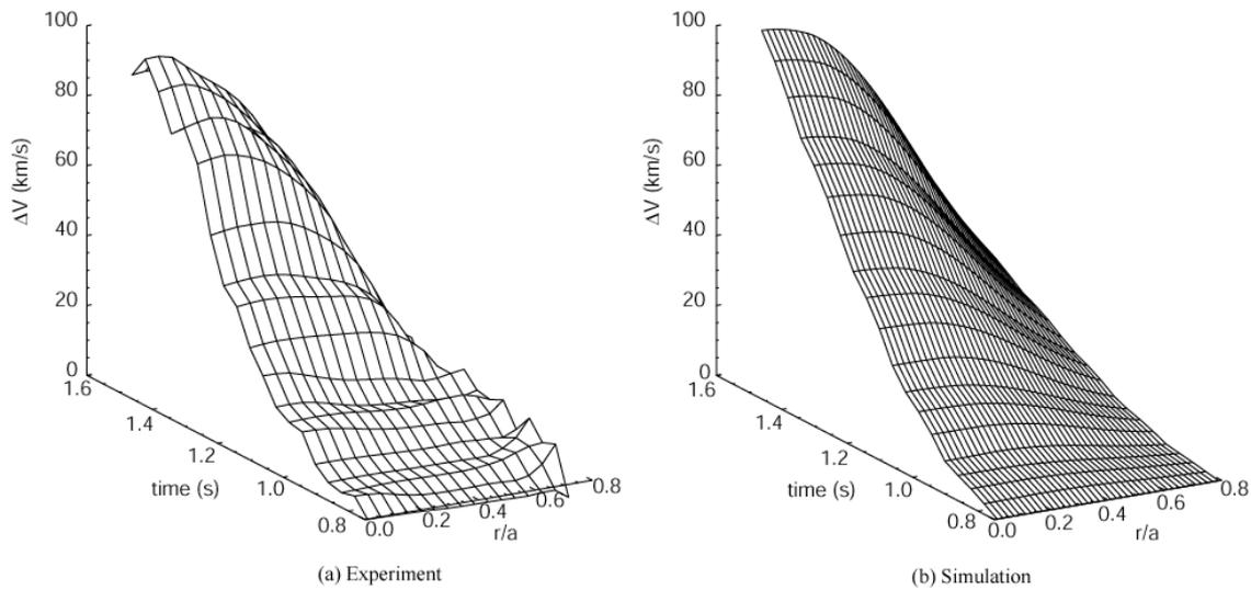
FIG. 6. Surface plots of  $\Delta V_\phi = V_\phi - V_\phi(P_{rf} = 0)$  vs.  $r/a$  and time for the MC plasma in Fig. 1. (a) Experimental data; (b) Momentum transport modelling.
