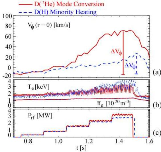
FIG. 1. (a) Central  $V_\phi$  after rf power application at 0.75 sec in an MC plasma (red solid) and an MH plasma (blue dashed); (b)  $T_e$  and  $n_e$  traces; (c) rf power traces.
