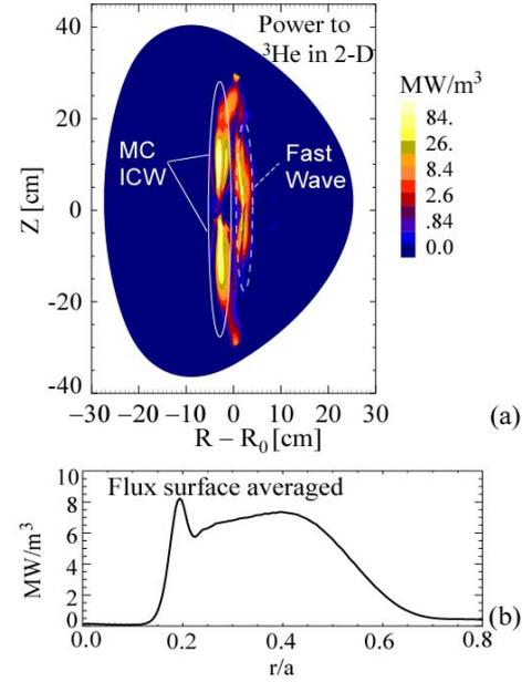
FIG. 5. TORIC simulation on MC ICW power deposition to  ${}^3\text{He}$  ions: (a) 2-D plot; (b) flux surface averaged.
