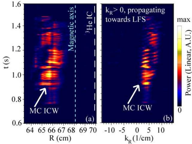
FIG. 4. MC ICW detected by PCI line integrated density fluctuation at the heterodyne RF frequency: (a) vs.  $R$  and  $t$ . (b) vs.  $k_R$  and  $t$ .
