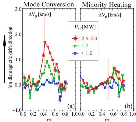
FIG. 3. Poloidal velocity profiles at different RF power levels: (a) MC plasma; (b) MH plasma.
