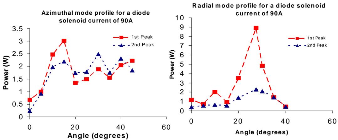
**Figure 3:** Antenna patterns recorded from the experiment when tuned for 11.7GHz resonance with a field of 0.03T on the cathode
