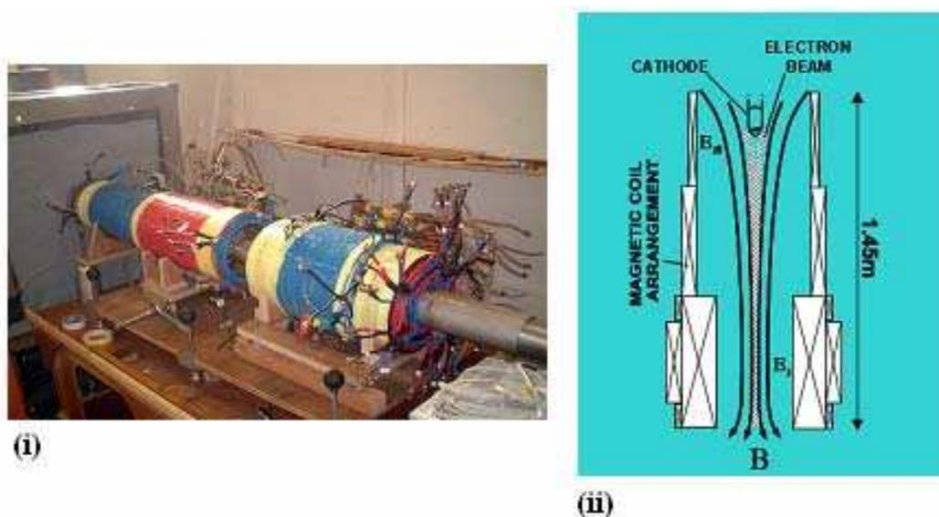
**Figure 1:**(i) Experimental and solenoid assembly (ii) Schematic of experimental apparatus.
