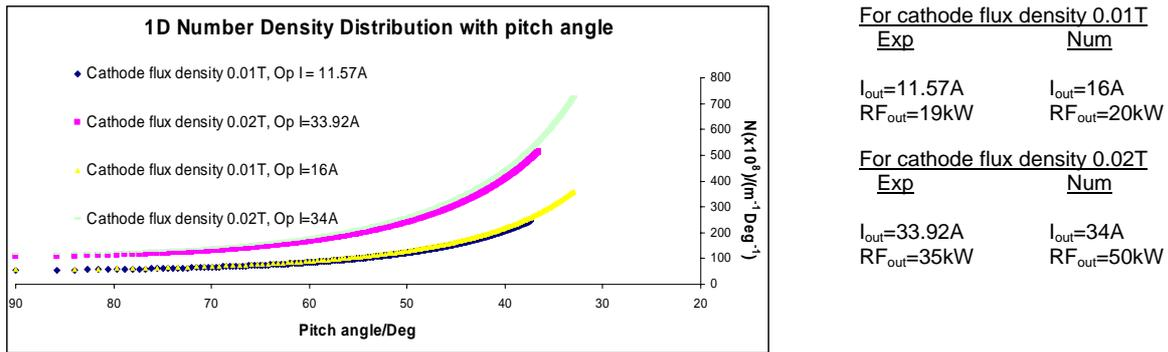
**Figure 2:** Illustration of the variation of electron density with pitch angle in both experiments (blue and magenta) and simulations for two different configurations of the electron injector; comparison of the predicted and measured RF output at 4.42GHz [9]
