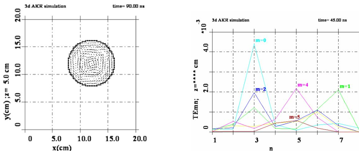
**Figure 4:** 3D PiC code predictions of the modes excited in the experiment at 11.7GHz showing the transverse E field pattern of a  $TE_{0,3}$  mode and the spatial Fourier analysis of the modes excited showing strong generation of the  $TE_{2,3}$  and  $TE_{0,3}$  modes
