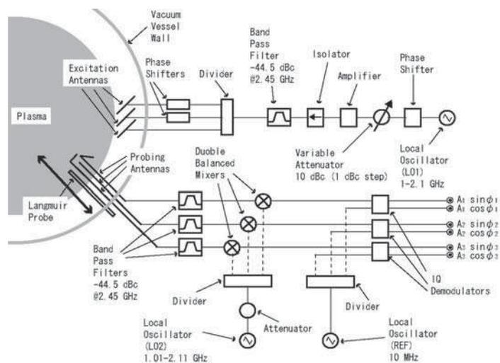
Fig. 1 Heterodyne method has been adopted, and IQ demodulators give cosine and sine (real and imaginary part) of signals. Band Pass Filters (BPFs) prevent penetration of microwave for heating.
