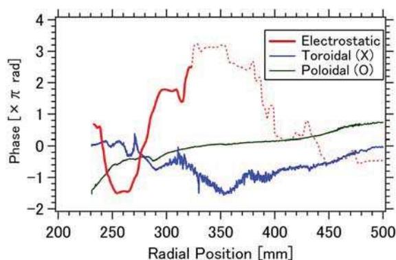
Fig. 3 Phase profiles of each component of an ECRF electric field.
