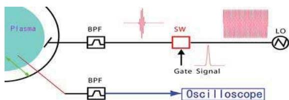
Fig. 5 Schematic drawing of pulse injection experiments.
