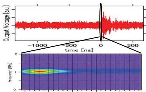
Fig. 6 Preliminary result of pulse arrival time.
