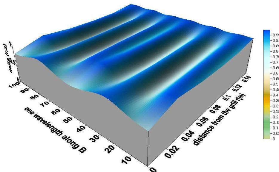
Fig. 1. Graph of  $\delta(r,z)$  for the LH power flux =  $1.86 \text{ kW/cm}^2$  (corresponds to 1.5 MW on C2),  $L_T=3 \text{ cm}$ ,  $L_n=1 \text{ cm}$ ,  $T=20 \text{ eV}$ ,  $n_b=2.4 \times 10^{17} \text{ m}^{-3}$ .
