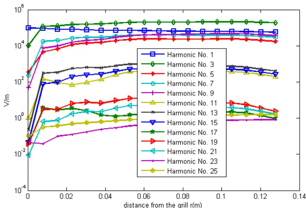
Fig. 5. The radial profile of higher spatial harmonics of the scattered field, propagating in the + direction, for the LH power  $1.24 \text{ kW/cm}^2$  (corresponds to 1 MW on C2).
