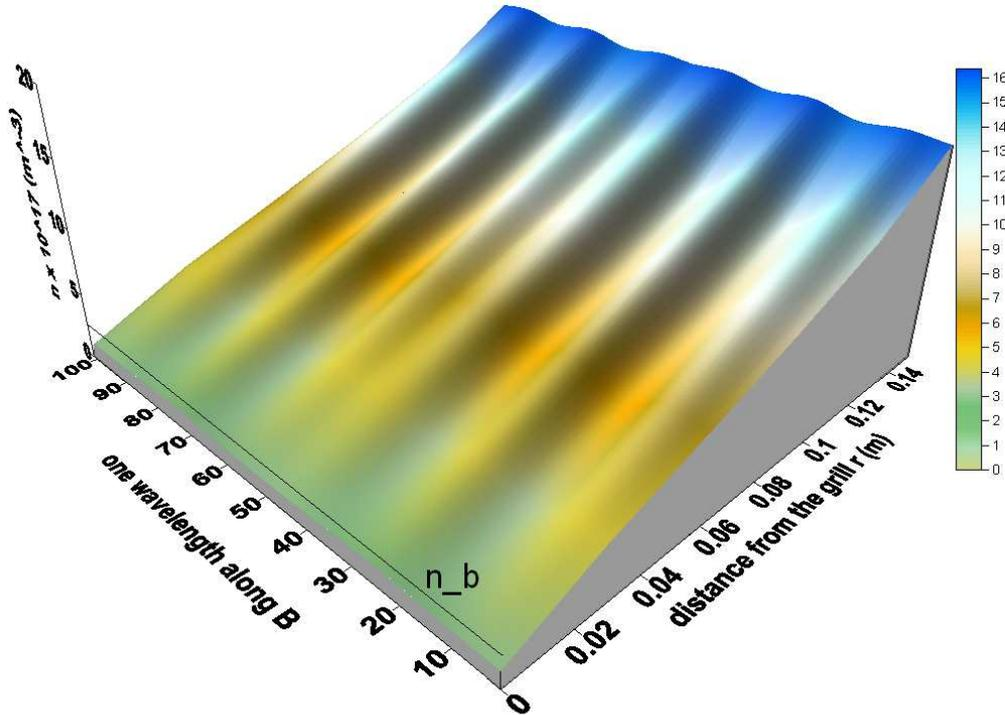
Fig. 2. Graph of  $n(r,z)$  for the LH power flux =  $1.86 \text{ kW/cm}^2$  (corresponds to  $1.5 \text{ MW}$  on C2),  $L_T=3 \text{ cm}$ ,  $L_n=1 \text{ cm}$ ,  $T=20 \text{ eV}$ ,  $n_b=2.4 \times 10^{17} \text{ m}^{-3}$ .
