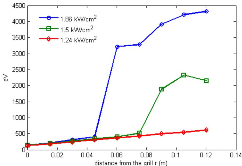
Fig. 3. Acceleration of electrons in the scattered field as a function of radius for varying LH power flux from 1.24 to 1.86 kW/cm<sup>2</sup> (corresponds to 1 - 1.5 MW on C2),  $L_T=3$  cm,  $L_n=1$  cm,  $T=20$  eV,  $n_b=2.4 \times 10^{17}$  m<sup>-3</sup>, the initial electron energy is 80 eV.
