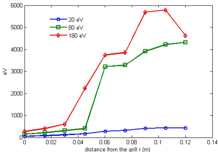
Fig. 4. Acceleration of electrons in the scattered field as a function of radius for the LH power 1.86 kW/cm<sup>2</sup> (corresponds to 1.5 MW on C2), and varying initial electron energy from 20 to 180 eV.
