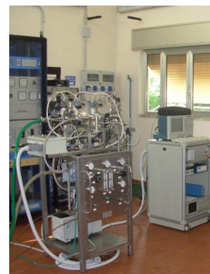
*Fig. 3. The automatic TSG facility for testing of valve components*
