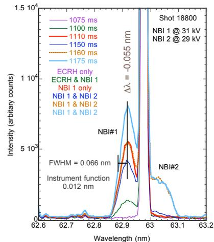
Fig 3: Features appear on the short and long wavelength sides of the O V line at 62.97 nm during NBI heating
