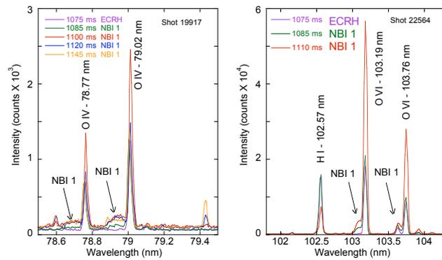
Fig. 4 Features appear on the short wavelength sides of O IV (79 nm) and O VI (103 nm) lines during NBI#1 heating.
