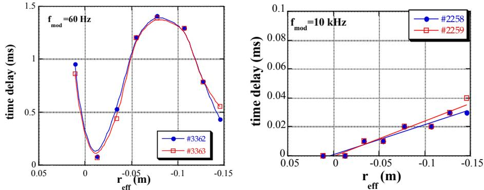
Figure 1: Time delay in several modulation experiments on TJ-II. a) Two shots with modulation frequency 60 Hz. b) Two shots with modulation frequency 10 kHz.
