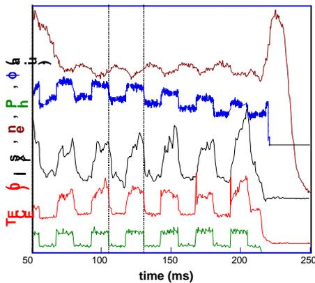
Figure 2: Time evolution of central potential and temperature, SXR intensity and line density in a discharge with  $f_{mod} = 40$  Hz and a modulated power of 200 kW over a 200 kW continuous heating power.
