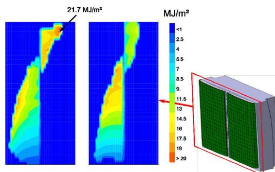
Fig. 1 b First wall shape and power load [3]
