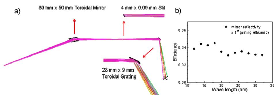
**Figure 3.** a) Ray tracing by ZEMAX program. b) Calculated efficiency.
