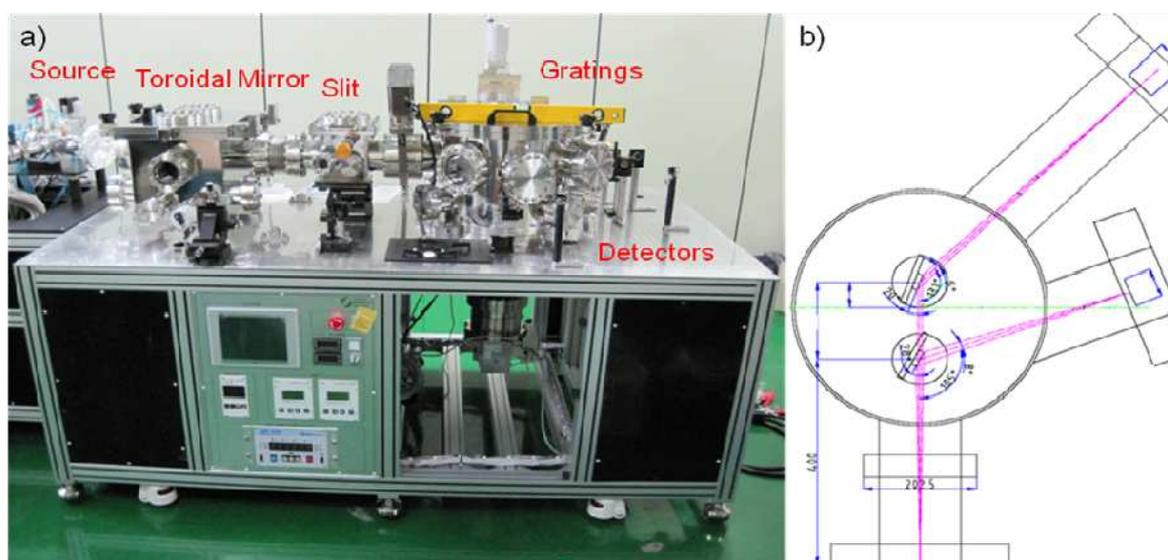
**Figure 1.** a) The VUV spectrometer prototype system. b) The top view of the grating chamber.
