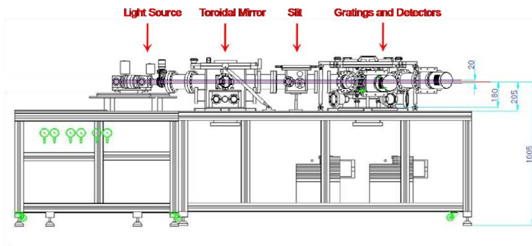
**Figure 2.** The front view. Height difference between gratings is 2 cm from center to center.
