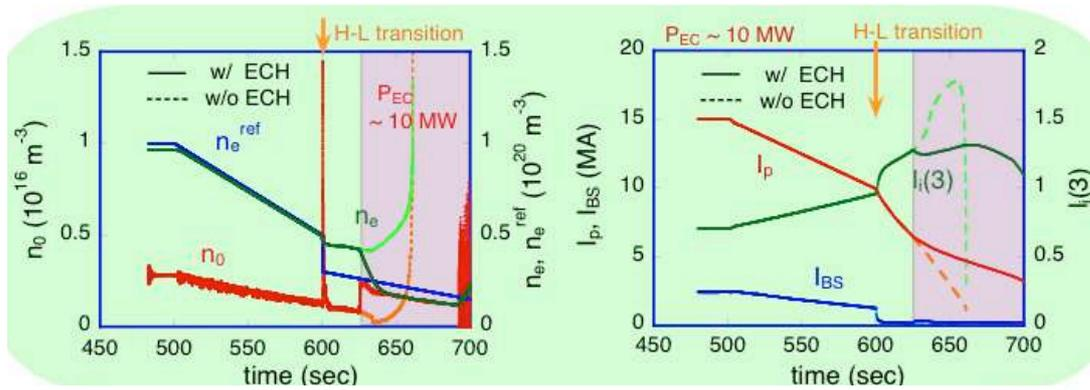
Fig. 3 Termination with pumping-performance degraded and avoidance of radiation collapse by means of O-mode ECH of  $P_{EC} \sim 10$  MW (solid lines). (1)  $n_e$ ,  $n_e^{ref}$  and  $n_0$ . (2) control performance of  $I_p$  ramp-down and evolution of  $l_i(3)$  ECH
