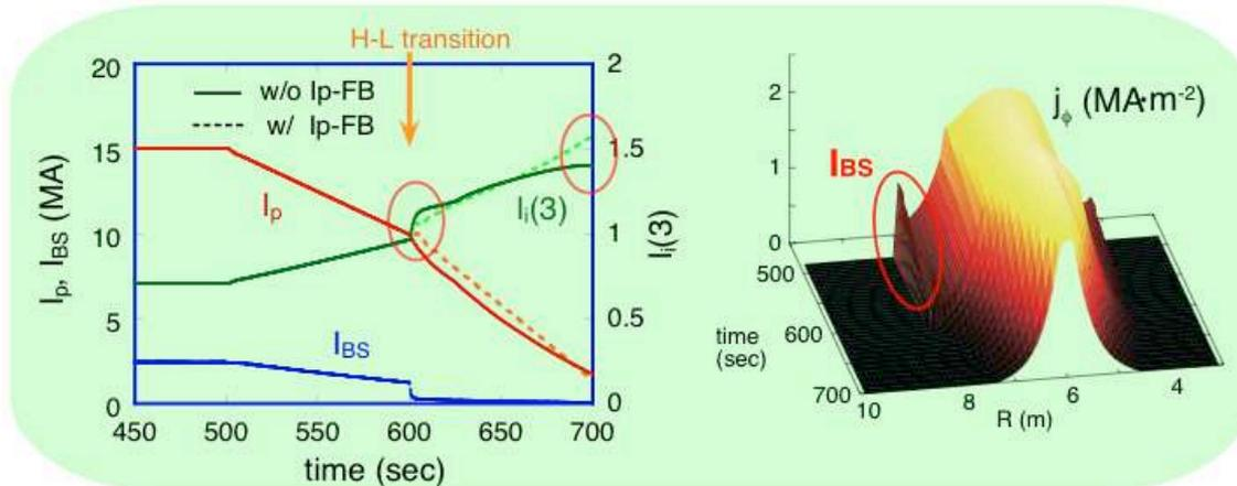
Fig. 2 Termination with pumping-performance enhanced. (1) control performance of  $I_p$  ramp-down and evolution of  $l_i(3)$ ; (2) plasma current profile
