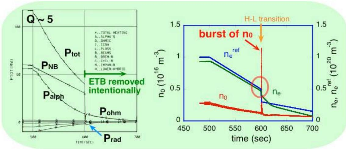
Fig. 1 Termination with pumping-performance enhanced. (1) Fusion power  $P_{\alpha}$ , NB heating power  $P_{NB}$ , total heating power  $P_{tot} (= P_{\alpha} + P_{NB})$ , ohmic heating power  $P_W$  and radiation power  $P_R$ ; (2) volume-averaged plasma density  $n_e$ , reference plasma density  $n_e^{ref}$  and neutral density  $n_0$  in vacuum region.
